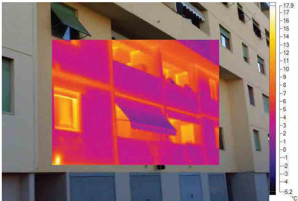
L'EDIFICIO RIQUALIFICATO NEL 2012 MOSTRA LA RISPOSTA TERMICA DI 2 MATERIALI DIFFERENTI UTILIZZATI PER LA FACCIATA NORD E LA FACCIATA OVEST. NELLA PRIMA IL CAPPOTTO TERMICO ASSICURA UNA BUONA TENUTA NONOSTANTE LA POSA IN OPERA NON RISULTI OTTIMALE. SULLA FACCIATA OVEST INVECE VENGONO MISURATI INVECE DIFFERENZE TERMICHE ESTREMAMENTE ELEVATI
